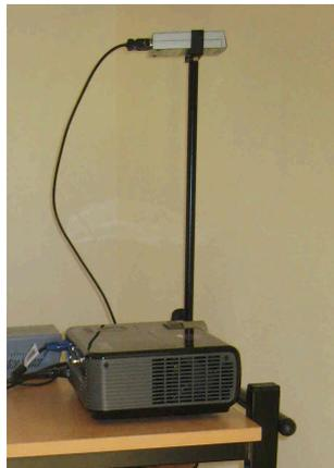
The infrared camera is mounted on a telescopic tube over the cart so that the pen is always in the field of vision of the camera.
